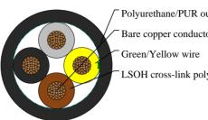
Polyurethane/PUR outer jacket Bare copper conductor LSOH cross-link polyolefin insulation
